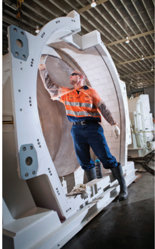
Applying WEAR MAX to centrifuge housing
